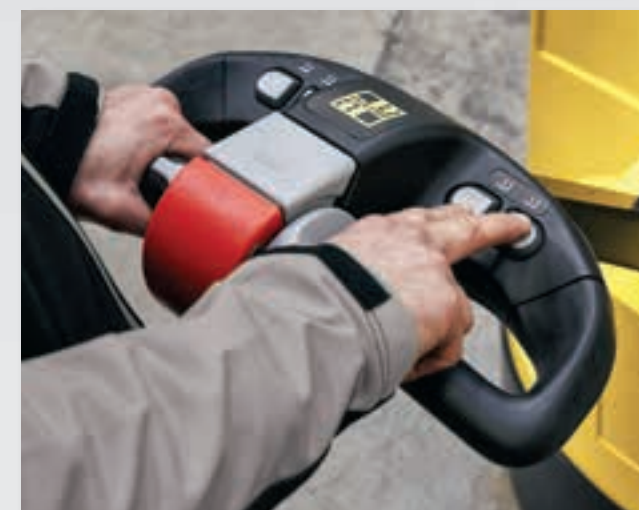
Ergonomically designed control handle.
